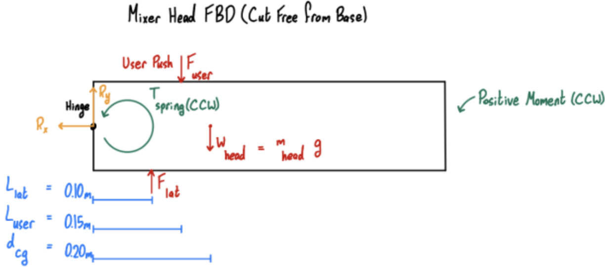
Figure H2: Free body diagram of the mixer head cut free from the base, indicating the head weight, latch force, user push, torsion spring torque, and the distances from the hinge to each of these forces.
